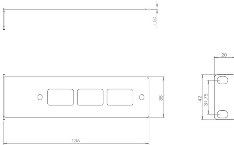
Attach and secure the brackets to the switch chassis with the provided screws and then rack mount the unit to the pillars of the rack, securing it with the rack's screws and cage nuts.
