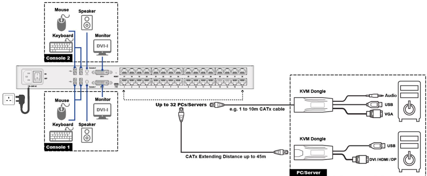
**Note:** S/FTP cable is recommended to provide protection against internal crosstalk, alien crosstalk, EMI, ESD and RFI.
