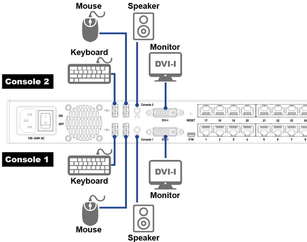
If you are connecting to an LCD Console Tray, use an appropriate video cable and USB 2.0 Type A Male – Type B Male cable to connect the ‘Console’ connectors to the LCD Console Tray (video converter or adapter may be required for different video interface).
